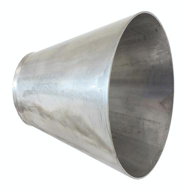
The cone bending process with the F series is simple. The bottom roll needs to be inclined to achieve cone bending geometry. This is controlled and monitored by electronic microprocessor. \*
